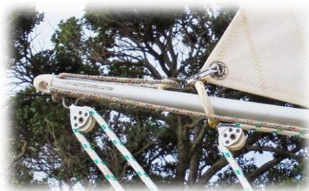
2. Unfurl the remaining sail by pulling on the starboard side of the reefing line until sail is fully unwrapped from the mast.
