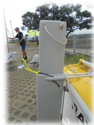
5. Fit the alloy joystick handle – this is best done after the sailor is seated, particularly when being craned in.
