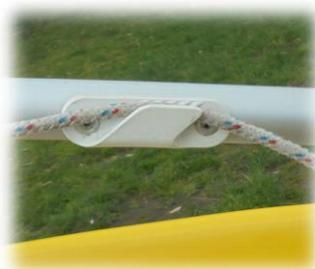
5. The idea is not to flatten the sail along the boom as it should have enough slack to form a gentle curve. This curve should be less in higher strength winds and more in light winds.
