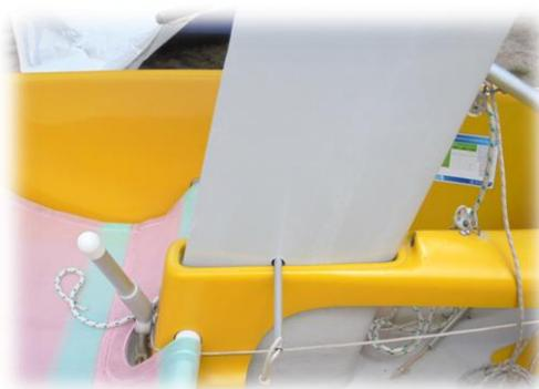
2. Launch the boat into the water on its trolley and float it clear – the trailer may float also, so you will need to push it down. Leave the centreboard pinned in the half way position if you need to move the boat around in shallow water or to a pontoon.
