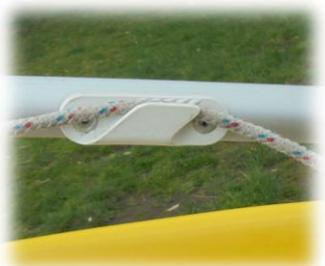
3. Pull on the port side of the reefing line to reduce sail area (You can generally put one complete turn of sail around the mast without adjusting the outhaul). To reef further the outhaul needs to be released to allow the sail to travel forward along the boom.
