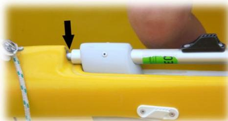
5. Slide the rudder blade into the rudder box with thicker edge facing forward, and ensure safety retainer bungee is across the top (if not done earlier).
