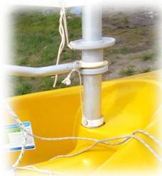
3. Sort out the thicker rope (the mainsheet), and shackle it onto the rope traveller which runs across the stern of the boat.
