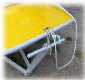
1. Use the short alloy tube to pin the centreboard up before launching or when moving the boat around onshore.
