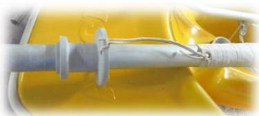
3. Haul the reefing line until the knot is positioned as far as it will go on the starboard (right hand) side - if the reefing line has been spliced to form a continuous loop this step is not necessary.
