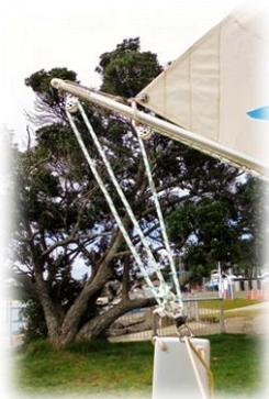
4. Pass the other end of the mainsheet through the block on the forward end of the console. Feed it through so it can be controlled from the seat.
