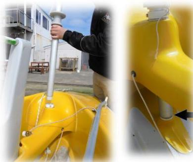
5. Reach under the console and tighten the knurled knob. This locks mast in place and tightens the reefing drum onto mast so that the sails can be reefed while sailing.
