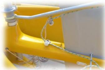
5. Tie a figure of eight knot on the end of the sheet to keep it in place.
