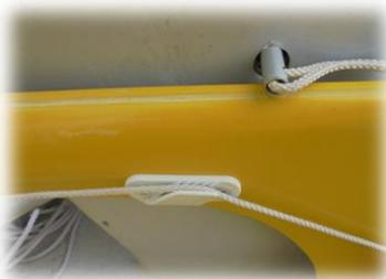
4. Pull the sail out to the end of the boom by pulling on the outhaul line then cleat the line at the front end of the boom.
